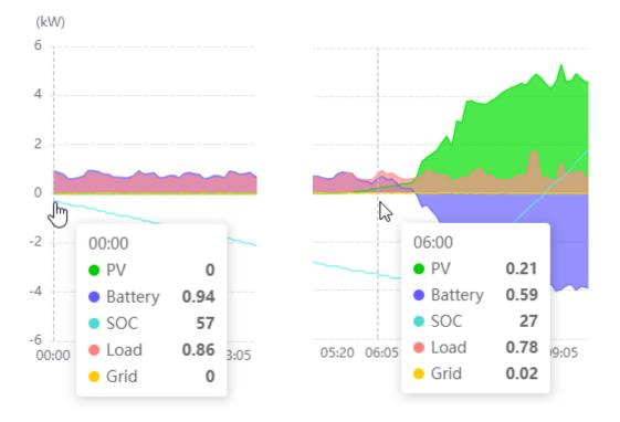
The SOC starts off at 57% at midnight and drops down to 27% at 6:00
