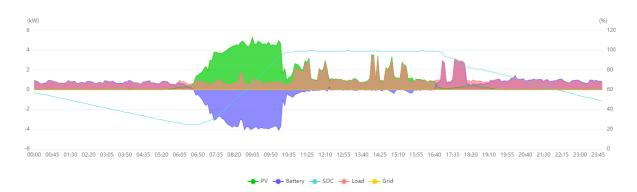
The system starts the day with the house load being supplied by the battery which has a SOC of 57% which gently drops to 25% at its lowest point
