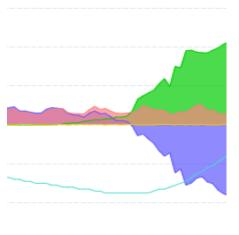
At 5:40 the solar starts to ramp up and starts to feed the house load with what it can generate, at the same time reducing the battery demand to the difference needed (reducing the dropping battery SOC significantly until it levels out at 25%)
