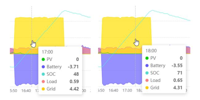
SOC increases from 48% to 71% = 23% increase in charge over 1 hour
