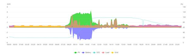
Sometimes the SOC will be close to the loadshedding SOC/V% when it hits the set period, in this case the battery is charged by the grid with a short burst to get it to the required level, and then it is maintained by the grid at that level until loadshedding starts
