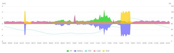
Note the use of battery to supplement solar between 9 and 11 am. If the battery SOC/V% was set to a high level for this period then the only option would be to use grid at that time
